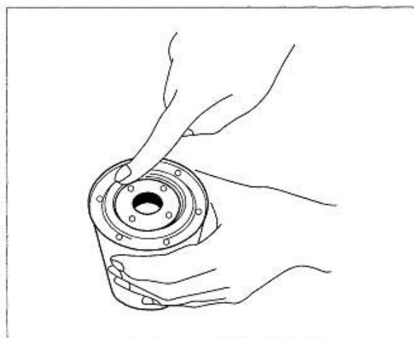
Figure 2-5 Replace Oil Filter Cartridge
