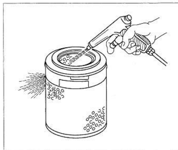
Figure 2-3 Clean the Air filter Cartridge
